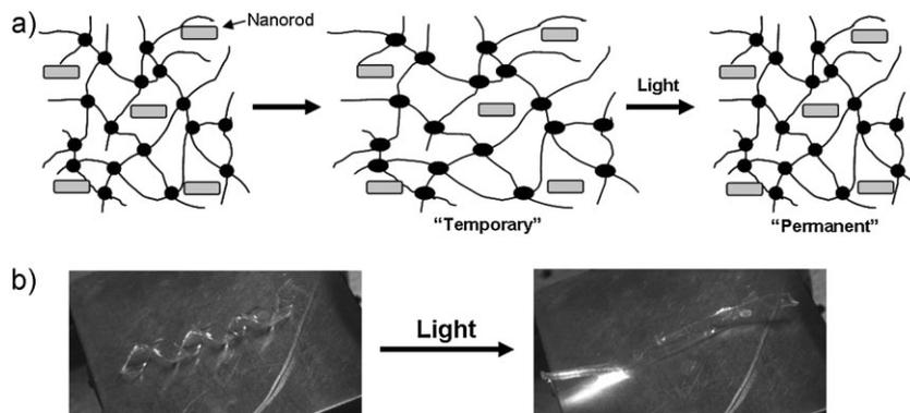
**Figure 4.** Light-induced transitions in shape-memory polymers. (a) Schematic of polymer network, where a material is heated above its  $T_g$  and set in a temporary shape and then cooled. UV light can then be introduced to heat the polymer via entrapped nanorods to again raise the temperature above the  $T_g$  to allow the material to return to its permanent shape. (b) Example of a coiled sample that returns to its rectangular shape with NIR light exposure.
